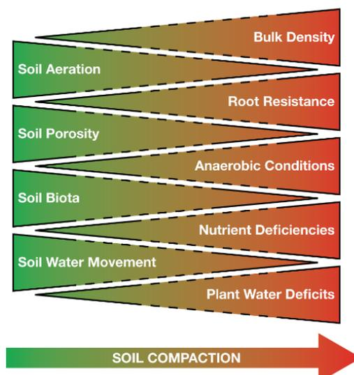
**Figure 4** Increasing or decreasing band widths indicate the likely effect of soil compaction on the soil property. Source: Hirons and Percival (2012).
