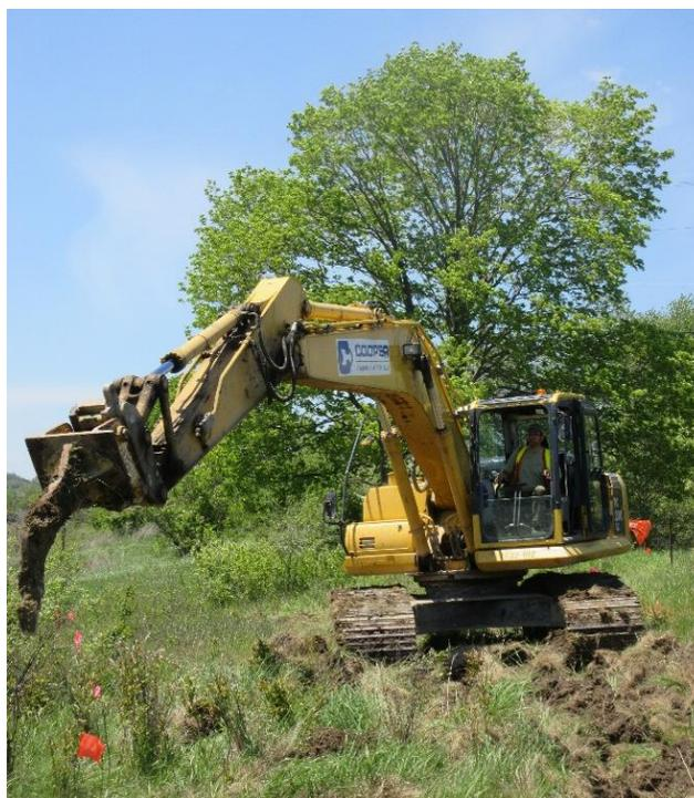
*Figure 10* An excavator with a ripping tine is effective for subsoiling compacted soils on larger sites.
