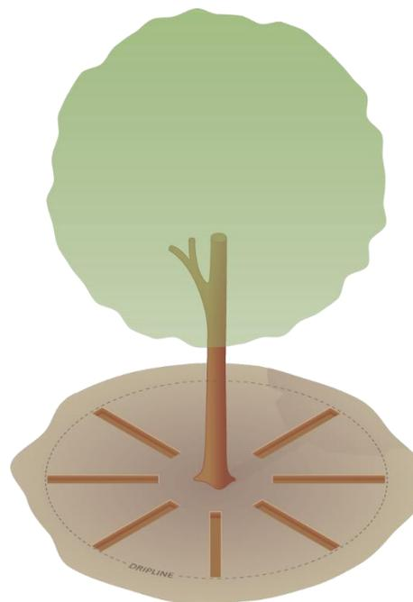
**Figure 12** In existing plantings or for new plantings where there is limited space to bring in equipment, radial trenching can be used to reduce compaction and increase organic matter. Radial trenching involves using air tools to excavate channels to the projected dripline and backfilling with mulch or other organic amendments. Source: Hiron and Thomas (2018).
