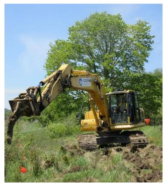
**Figure 10** An excavator with a ripping tine is effective for subsoiling compacted soils on larger sites.
